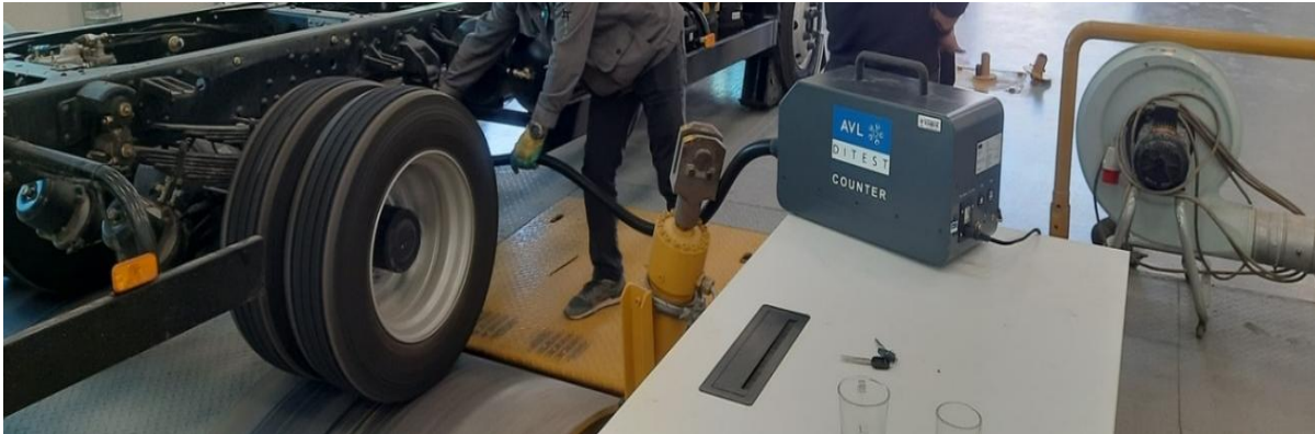
Figure 3: Device for measuring emitted particulate matter
