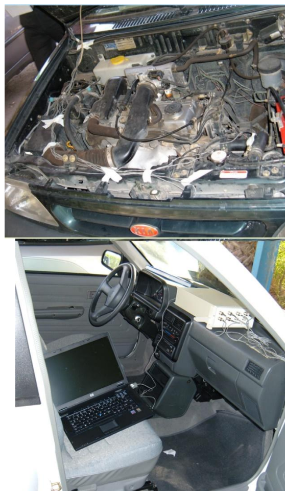
Figure 7: The data acquisition system and temperature sensors
