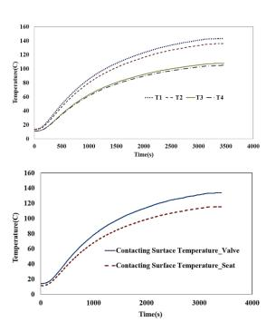
Figure 7: a) Measured sensors temperatures b) Contacting surfaces temperature
