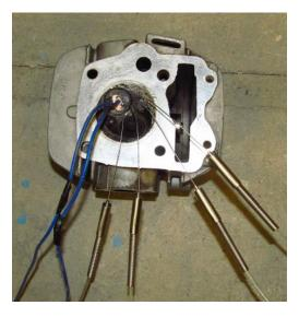
Figure 2:Thermocouples and heater installation [10]
