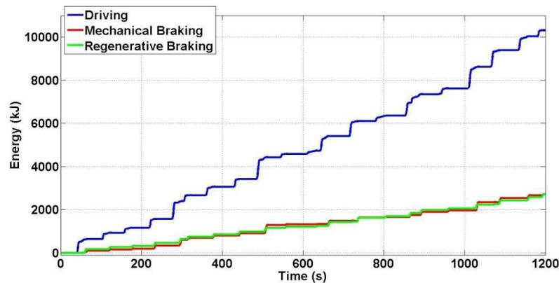
Fig10. Changes in driving, mechanical braking and regenerative braking energies using non-fuzzy control strategy
