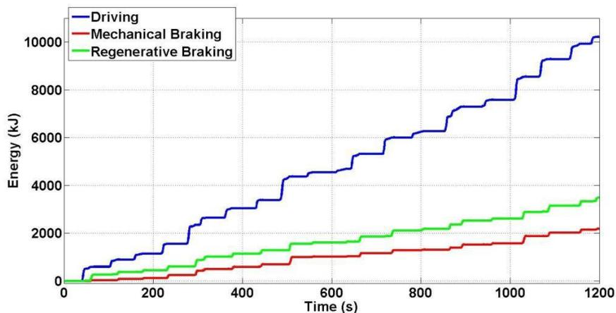
Fig11. Changes in driving, mechanical braking and regenerative braking energies using non-fuzzy control strategy
