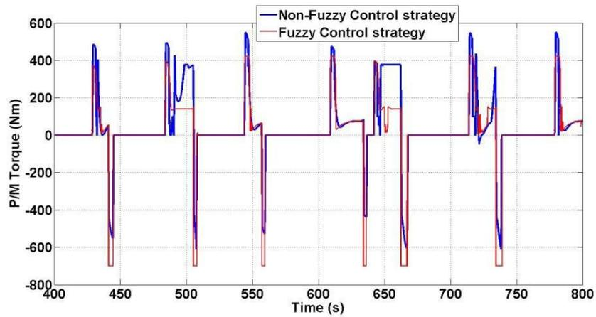
Fig13. Comparison of P/M command torque using fuzzy and non-fuzzy control strategy
