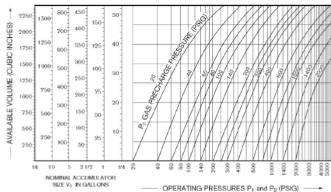
Fig7. Map of Volume-Pressure for Bladder Type Accumulator
