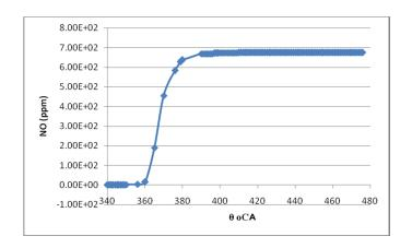
Fig4.NO emission from simulation results
