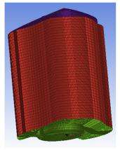
Fig1. Engine mesh generated in ICEM-CFD
