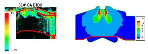
Fig3. equivalence ratio contours results in comparison to experimental
