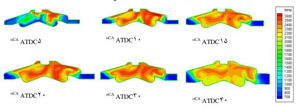
Fig5. Incylinder temperature contours
