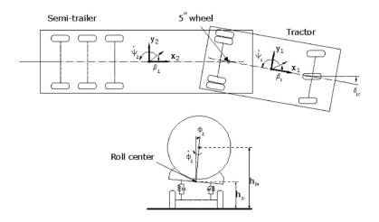
Fig1. Yaw and roll motion of tractor semi-trailer
