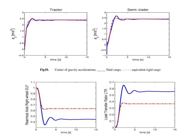
Fig11. Rearmost Axle Right wheel Dynamic Load Factor and Load Transfer Ratio; — fluid cargo, - - - - equivalent rigid cargo
