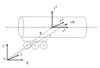
Fig3. Schematic diagram of the tank showing the moving and fixed coordinate frames
