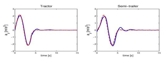
Fig15. Center of gravity accelerations; —— fluid cargo, - - - - equivalent rigid cargo
