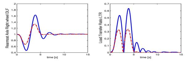
Fig16. Rearmost Axle's right wheel Dynamic Load Factor and Load Transfer Ratio; — fluid cargo, - - - - equivalent rigid cargo
