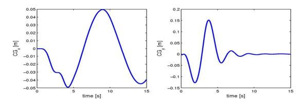
Fig13. Fluid's center of gravity coordinates (longitudinal and lateral)
