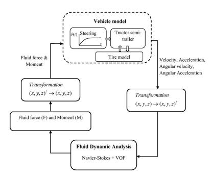
Fig4. Simulation procedure of fluid dynamics coupled with vehicle model
