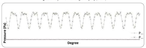
Fig10. Pressure versus the degree of gear rotating in the points Q (before gears) and R (after gears)
