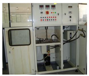
Fig16. Test setup of external gear pump
