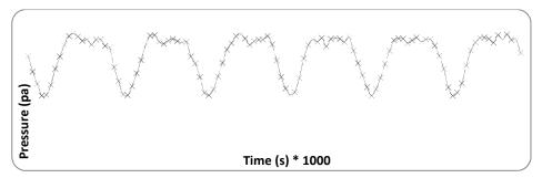
Fig11. Pressure versus the time of gear rotating in the point R in duration of a complete revolution
