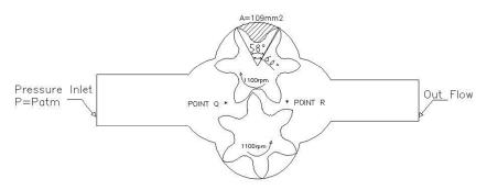
Fig9. Geometry of the modified gear oil pump (6 teeth)
