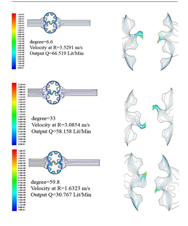
Fig17. Velocity contours (m/s) in the 3 divided parts of a gear rotating cycle
