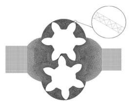
Fig7. Grid generation in physical domain
