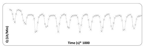
Fig14. Outlet displacement volume rate versus the time of gear rotating in duration of a complete revolution
