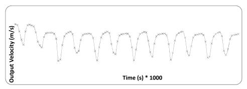
Fig13. Velocity versus the time of gear rotating in the point R in duration of a complete revolution
