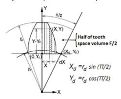
Fig6. The Schematic diagram of an involute tooth for calculating the space tooth
