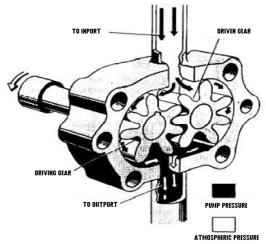
Fig1. Schematic diagram of main external gear pump with 7 teeth [1]
