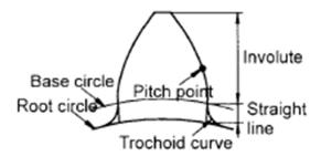
Fig4. Diagram of an involute tooth profile
