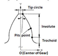
Fig5. Coordinate system of an involute tooth profile
