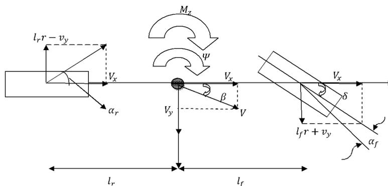
Fig3. Two-degree of freedom vehicle lateral dynamic model [18]
