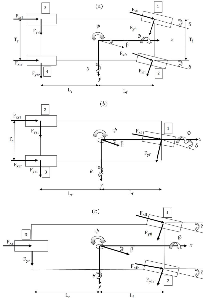
**Fig1.** (a) the fourteen-degree-of-freedom model for four-wheeled vehicle, (b) the twelve-degree-of-freedom model for three-wheeled car with front single wheel, (c) the twelve-degree-of-freedom model for three-wheeled car with rear single wheel
