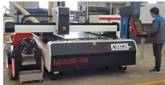
Figure 1: ACCURL laser tube cutting machine in operation
