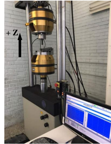
Figure 1. Fatigue test with Instron machine in Z direction.
