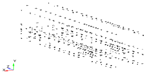
Figure 4: Bus rigid welding RBE2
