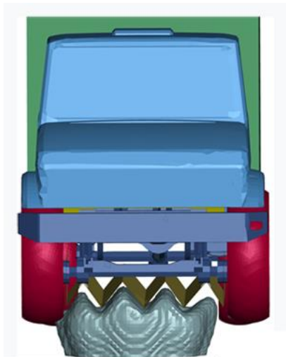
Fig. 6. Schematic view of Explosive device dispersion at 2.5ms.
