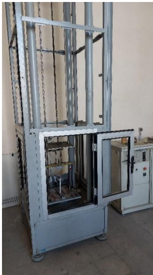
Figure 8: DCB impact test setup.
