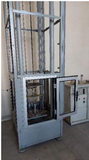
Figure 8: DCB impact test setup.
