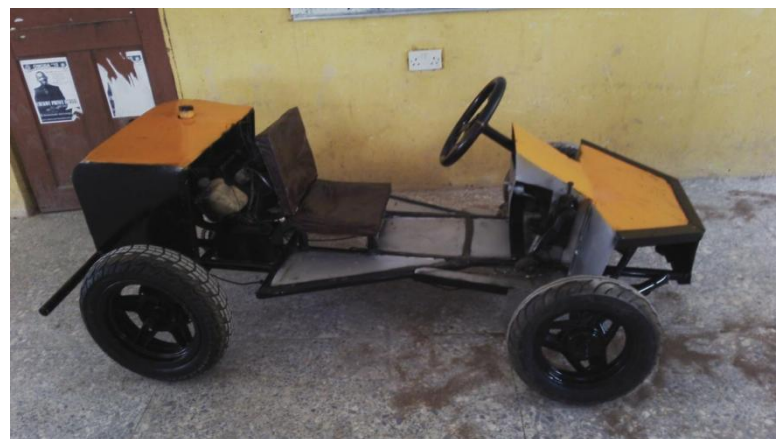
Figure5: Constructed Racing Go-Kart
