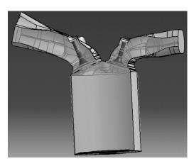
Fig 1. The geometry of the model designed for a diesel engine.
