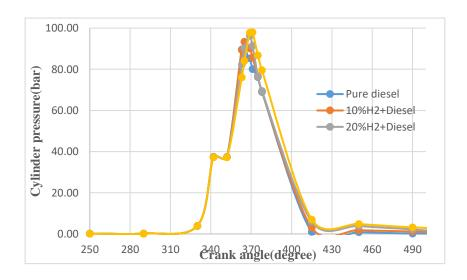
Fig 6. Variation of cylinder pressure versus crank angle with adding hydrogen to diesel fuel
