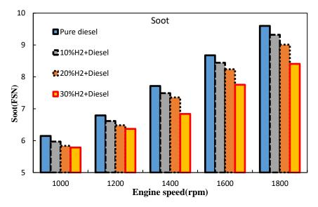
Fig 10. Variation of soot emissions versus engine speed with adding hydrogen to diesel fuel Automotive Science and Engineering
