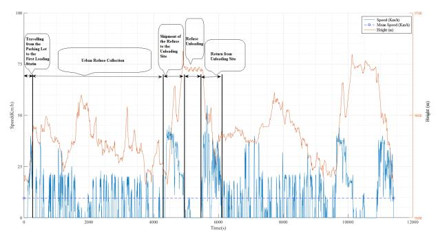
Figure 4: Speed and height versus time graph of refuse collection truck within half a working day
