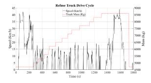
**Figure 6:** Generated refuse truck driving cycle together with the truck mass
