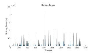
**Figure 7:** Braking power in Tehran refuse collection truck
