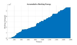
**Figure 8:** Accumulative braking energy in Tehran refuse collection truck.
