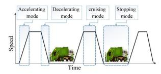
Figure 1: Pattern of the refuse collection driving cycle
