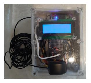
Figure 3: Data acquisition system
