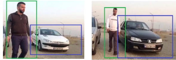
Figure 9: The human moving object with a green box and a vehicle moving object with a blue box are shown
