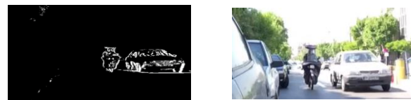
Figure 3: The right image is the initial image of the camera and the left image is the detection image of the moving objects
