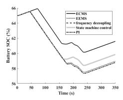
Fig.14. Battery SOC on different schemes with considering temperature variations (The ambient temperature=25 °C)
