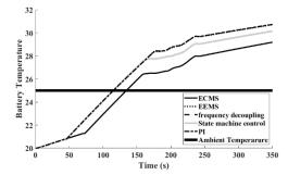
Fig.18. Battery temperature on different schemes with considering temperature
