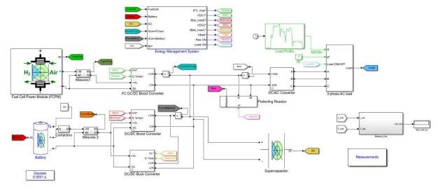
Fig.6. Case study: Example of fuel cell EMS
