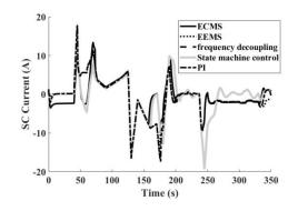
Fig.16. SC current on different schemes with considering temperature variations (The ambient temperature=25 °C)
