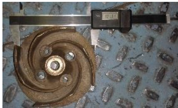
Figure 3: View of the pump's impeller
