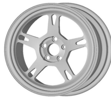
Figure 20: The optimized design after topology optimization
