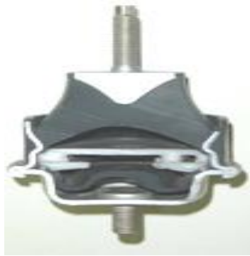
Fig24. Hydraulic engine mount with Inertia track
