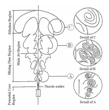
Fig1. Transient gaseous jet structure[33]
