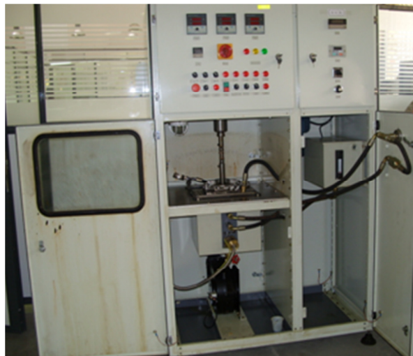
Fig16. Test setup of external gear pump
