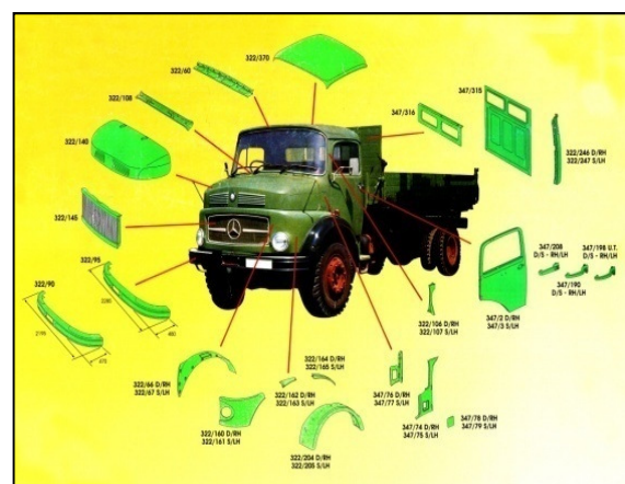
Fig5. Different parts of ECE-R29 truck cabin
