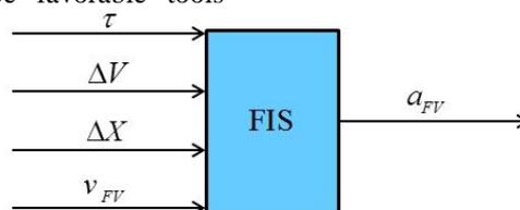
Fig3. Designed ANFIS model for car-following behavior.
