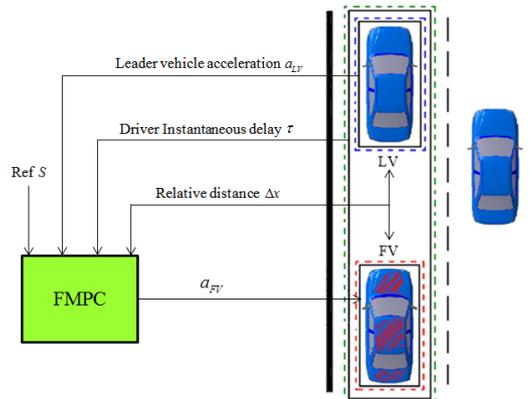
Fig5.Schematic of the ANFIS control system closed-loop
