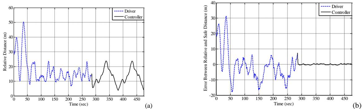
**Fig11.** performance of the FMPC system for car following behavior in comparison to the human driver, (a) relative distance between LV and FV, (b) relative distance error based on pipe rule
