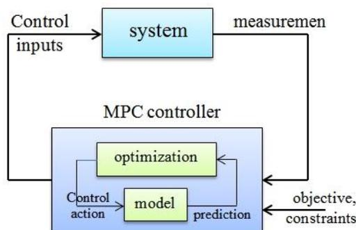
Fig2. Schematic representation of MPC [13].
