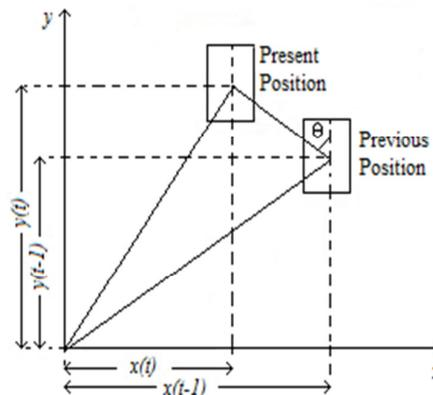
Fig7. The movement angle of the overtaking vehicle.
