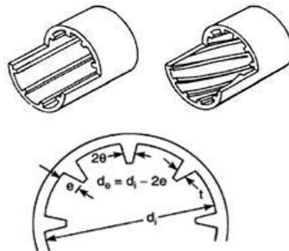
Fig5. Dimensional parameters for the fins [22]
