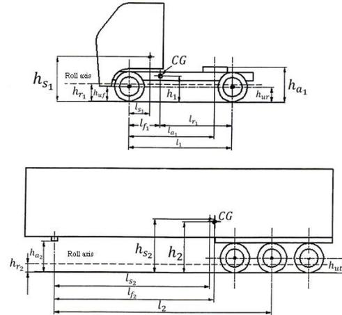
Fig2. Parameters of the articulated vehicle
