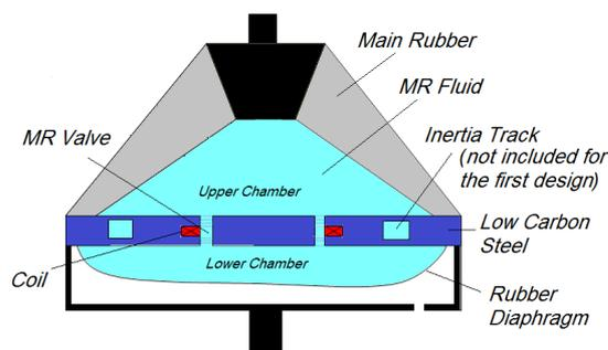
Fig. 2. Schematic of the MR engine mount
