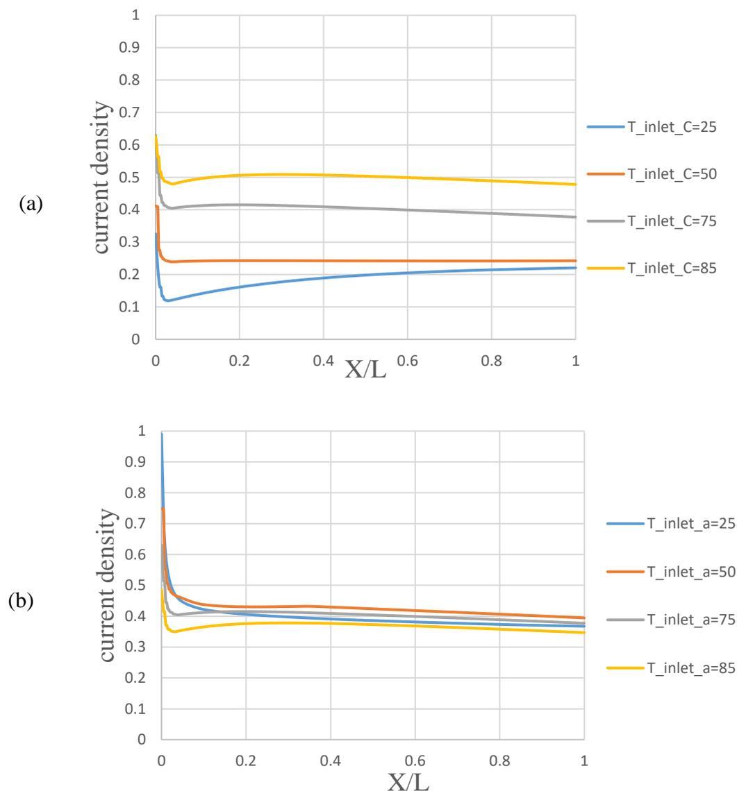
Fig.5. Current density of PEM fuel cell in different inlet temperatures. (a)Cathode side of PEMFC (b) Anode side of PEMFC
