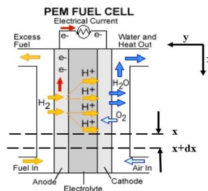
Figure 1. View of a cell in a PEM fuel cell.
