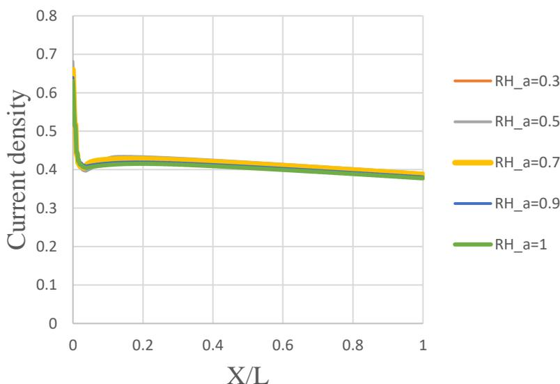
Fig.4. Current density of PEM fuel cell in different relative humidity. (a)Cathode side of PEMFC (b)Anode side of PEMFC
