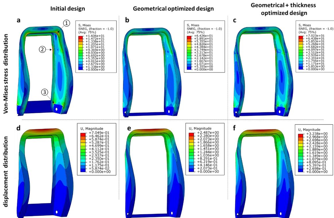
**Figure 7:** Simulation results of the Mg alloy seat frame in the backrest moment test (a-c) von-Mises stress and (d-f) displacement distribution.
