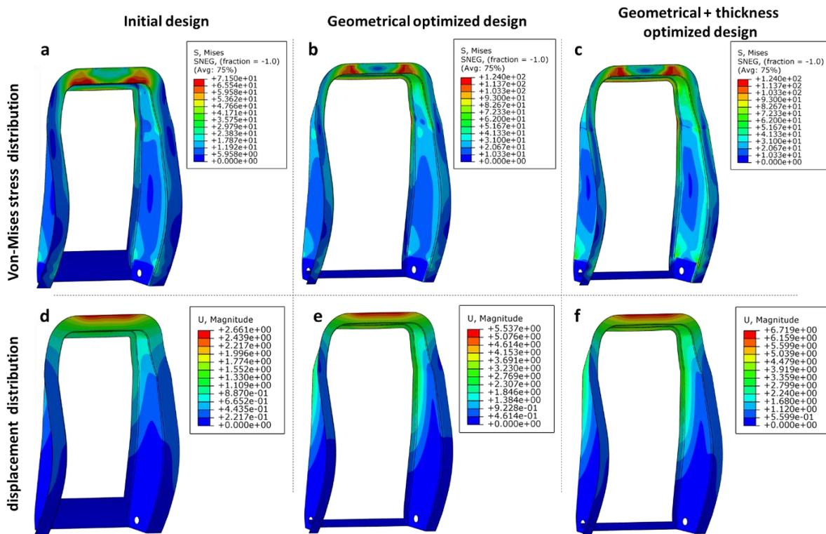
Figure 8: Simulation results of the Mg alloy seat frame in the static strength headrest test (a-c) von-Mises stress and (d-f) displacement distribution
