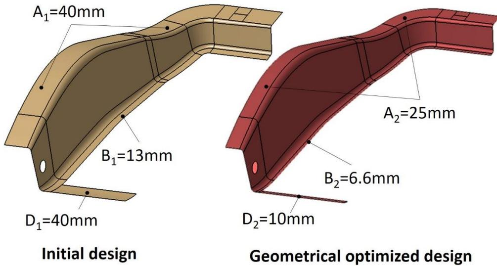
**Figure 4:** The initial and the geometrical optimized designs of the Mg alloy backrest
