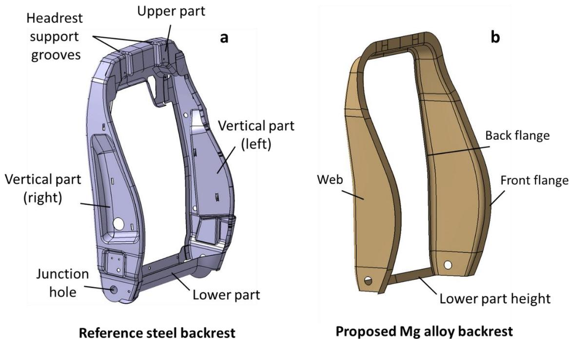
**Figure 1:** CAD drawing of the (a) reference steel backrest and (b) the proposed Mg alloy backrest
