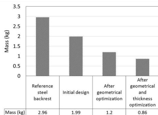
**Figure 9:** Weight reduction of the backrest from steel to Mg alloy and by two steps of optimization
