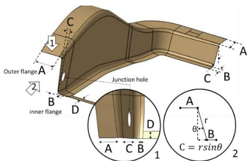
**Figure 3:** Geometrical optimization variables in the proposed Mg backrest
