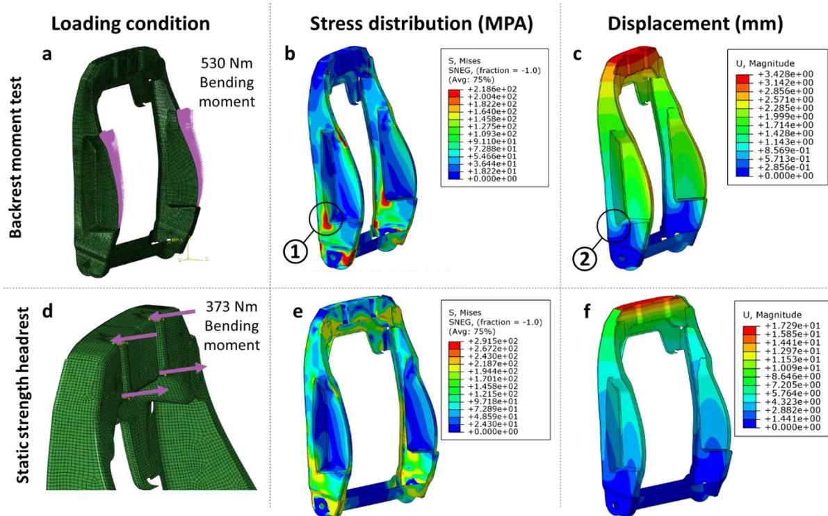
**Figure 2:** Loading conditions, stress and displacement distribution on the steel reference backrest
