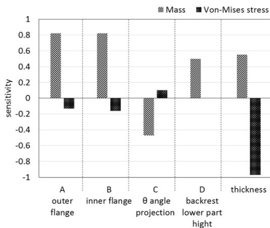
**Figure 5:** Sensitivity of different geometrical dimensions on the backrest mass and the maximum stress
