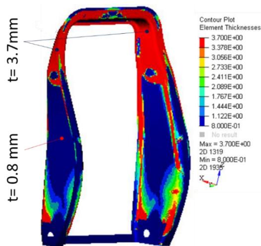
**Figure 6:** Thickness distribution of the Mg alloy backrest after shape optimization stage.
