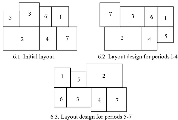
Fig. 6. Flexible machine layout design for P7
