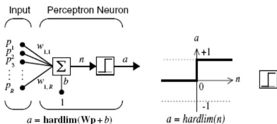
Fig. 4. A perceptron neuron with hard-limit function
