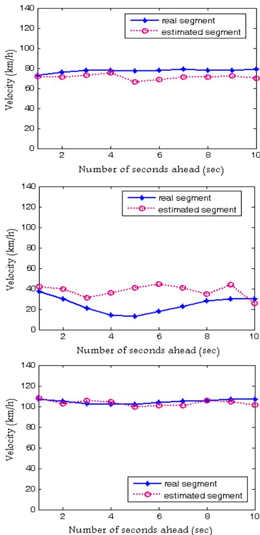
Fig. 9. three sample 10-sec segments predicted using neural networks
