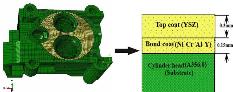
Fig2. The FE model of the coated cylinder head
