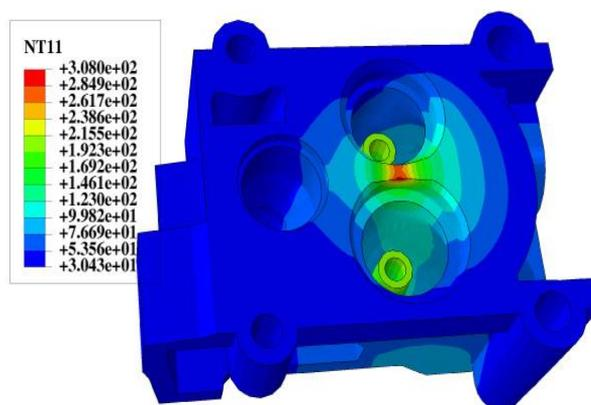
Fig3.. The temperature distribution in the uncoated cylinder head
