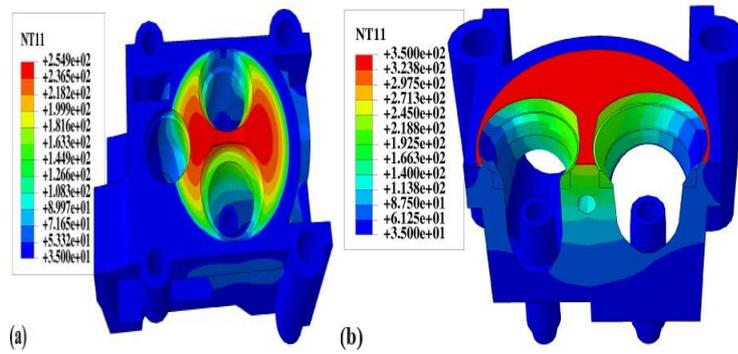
Fig4. The temperature distribution in the coated cylinder head: (a) without TBC, (b) with TBC
