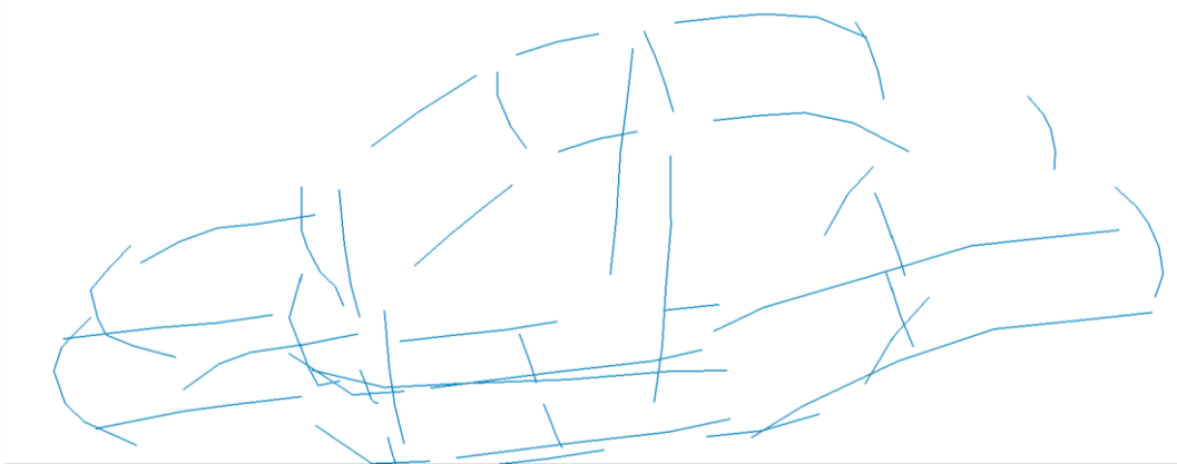
Fig3.: Equivalent beam modeling of the BIW
