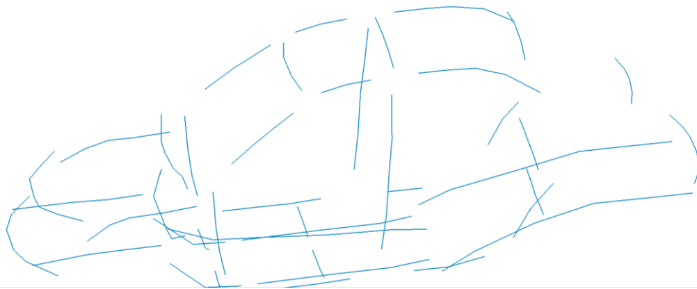
Fig3.: Equivalent beam modeling of the BIW
