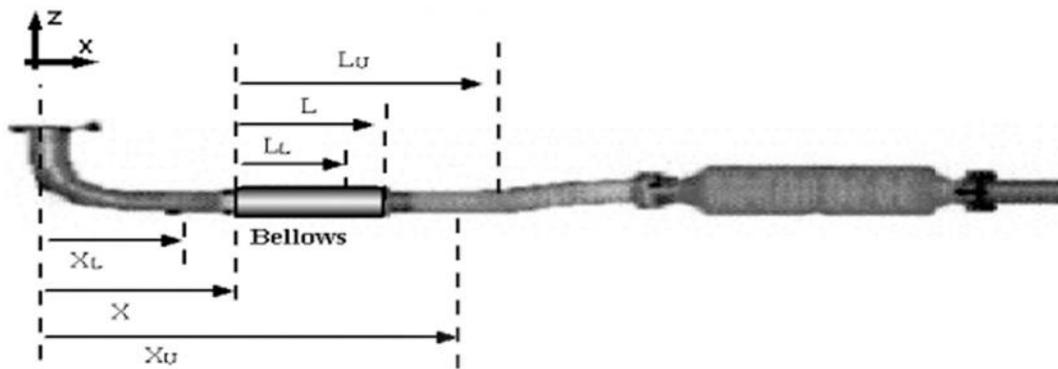
Figure 11: Optimization of position and length of Bellows
