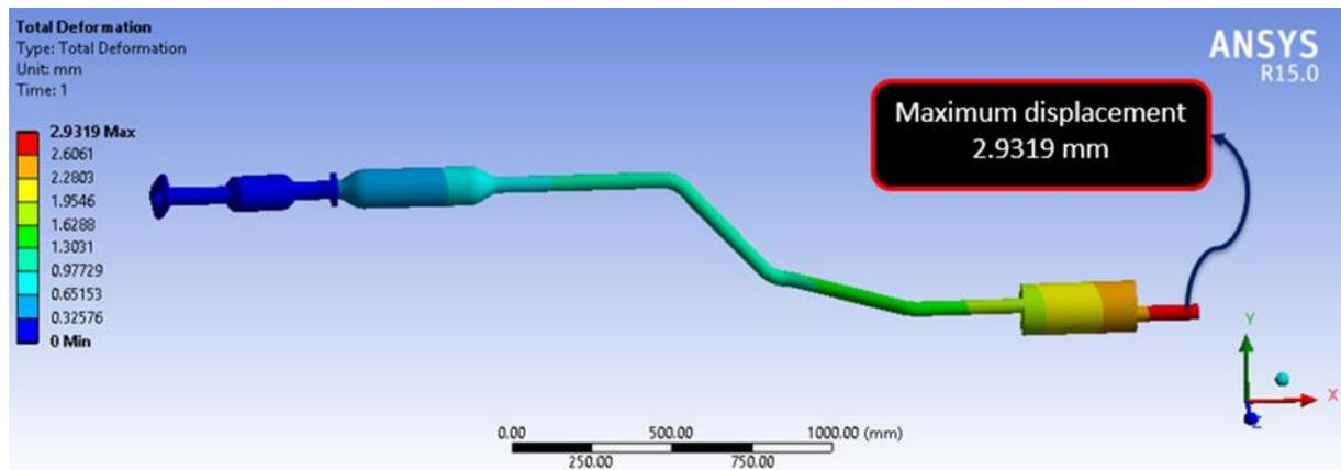
Figure 8: Maximum displacement of the exhaust system
