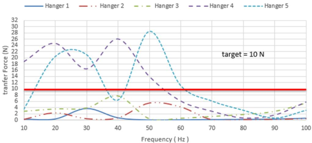
**Figure 10:** Transmitted forces at the hanger location
