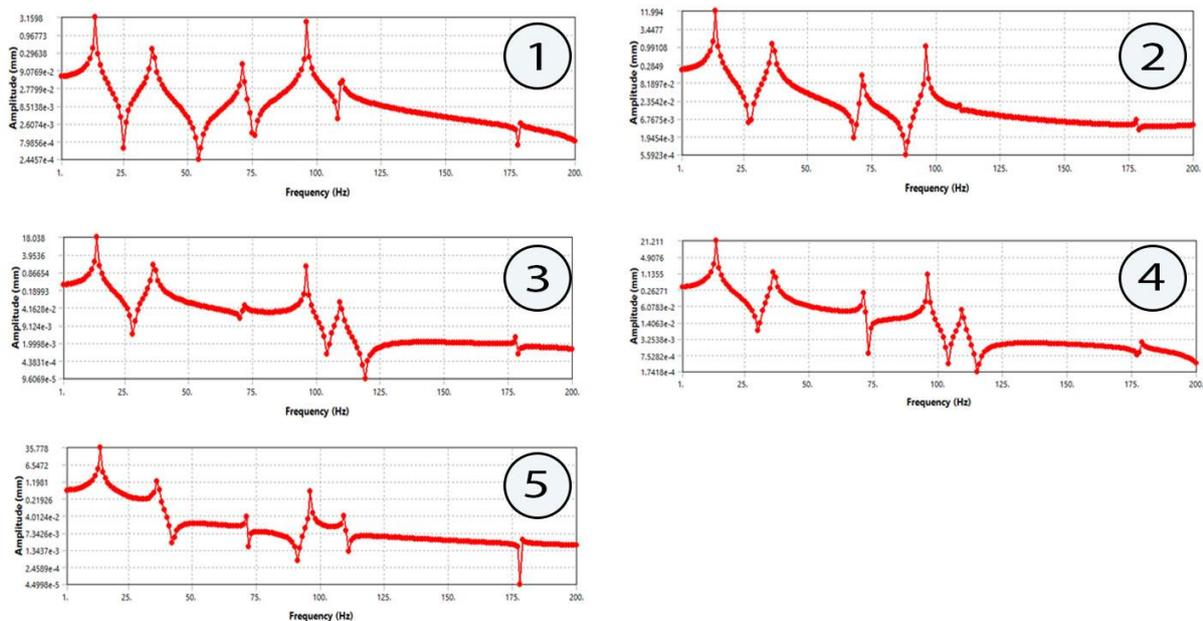
Figure 9: Characteristic displacement-frequency response for suspension point 1 to 5
