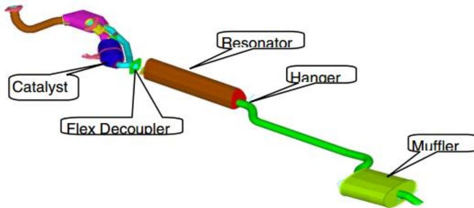
Fig1.: Schematic representation of an exhaust system
