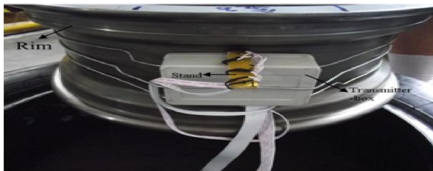
Fig1. The radio transmitter system placed inside the tire which is presented by Huang et al.[18].
