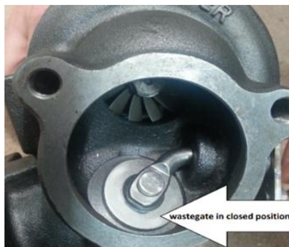
Fig6. Position of waste gate valve in the closing state.
