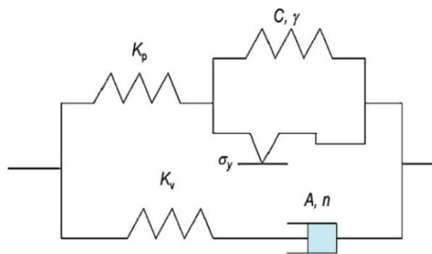
Fig4. The two-layer viscoelasticity model [32].
