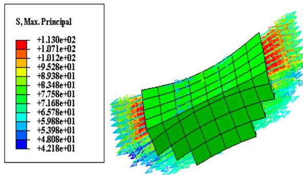
Fig14. The maximum principal stress vectors in the valve bridge when engine shuts off (in thirtieth second).
