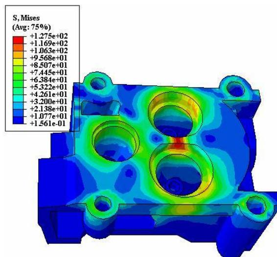
Fig9. The Von-Mises stress distribution at the end of the second stage of mechanical loading.
