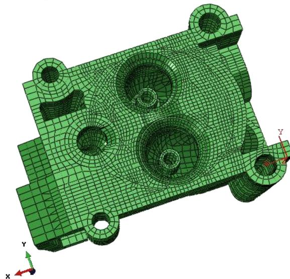
Fig5. The meshed cylinder head [38].
