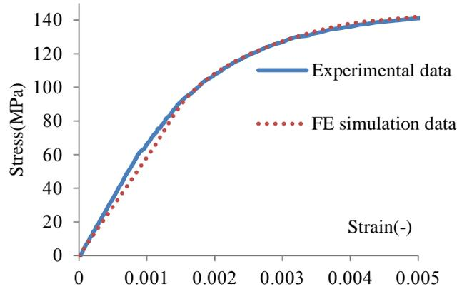
Fig6. Stress-strain behavior in tensile test of A356.0 alloy at 25°C.
