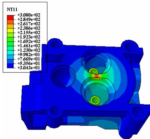
Fig10. The temperature distribution in the cylinder head[39].
