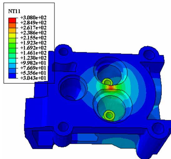
Fig8. The temperature distribution in the cylinder head.
