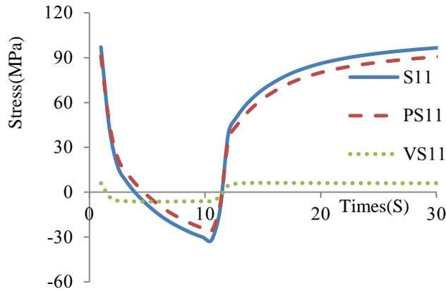
Fig12. The normal, plastic and viscous stresses in the X direction for point 1 of element 50152 versus time.
