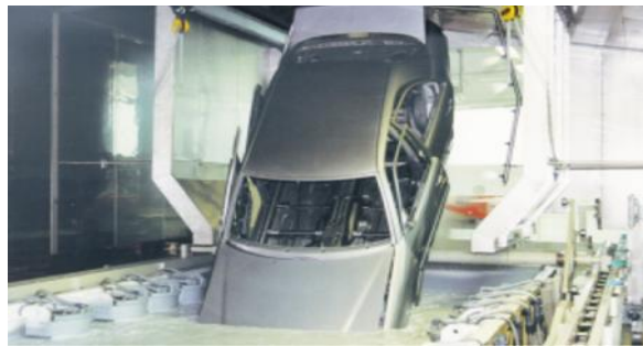
Fig. 1 Automobile in ED-coating step
