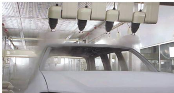
Fig.2 Painting of the exterior part of the body by robot
