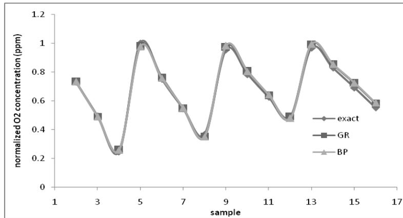
Fig10. Comparison of O<sub>2</sub> concentration predictions by GR and BP neural networks with experimental data for B10.
