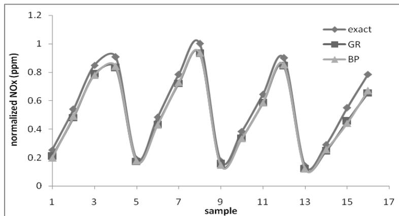
Fig12. Comparison of NO<sub>x</sub> emission predictions by GR and BP neural networks with experimental data for B10.
