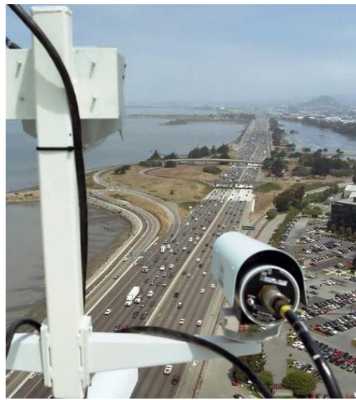
Fig3. A digital video camera mounted on top of a building that overlooks I-80 is recording vehicle trajectory data [14]
