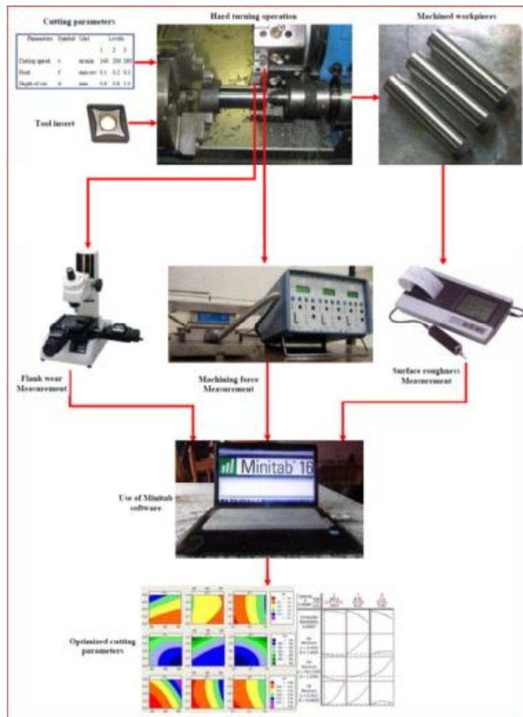
**Fig1.** Experimental setup
