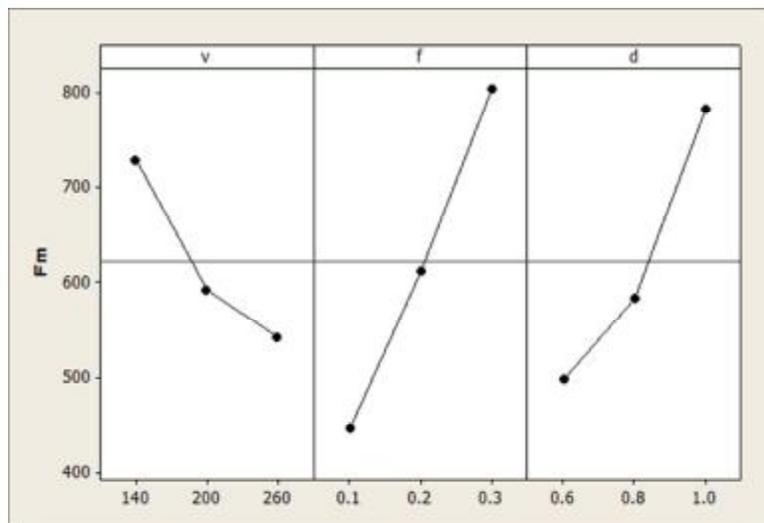
Fig3. Main effect plots for machining force (Fm)
