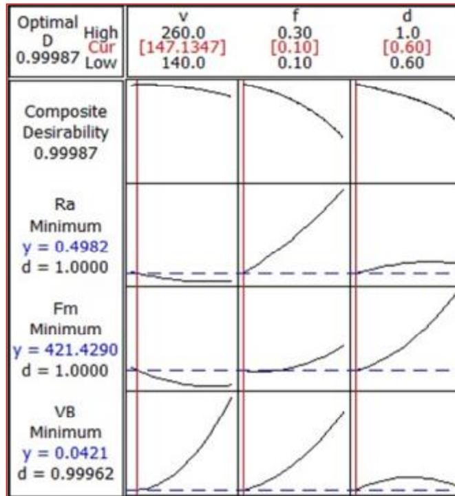
Fig6. Response optimization plot for surface roughness (Ra), machining force (Fm) and flank wear (VB)
