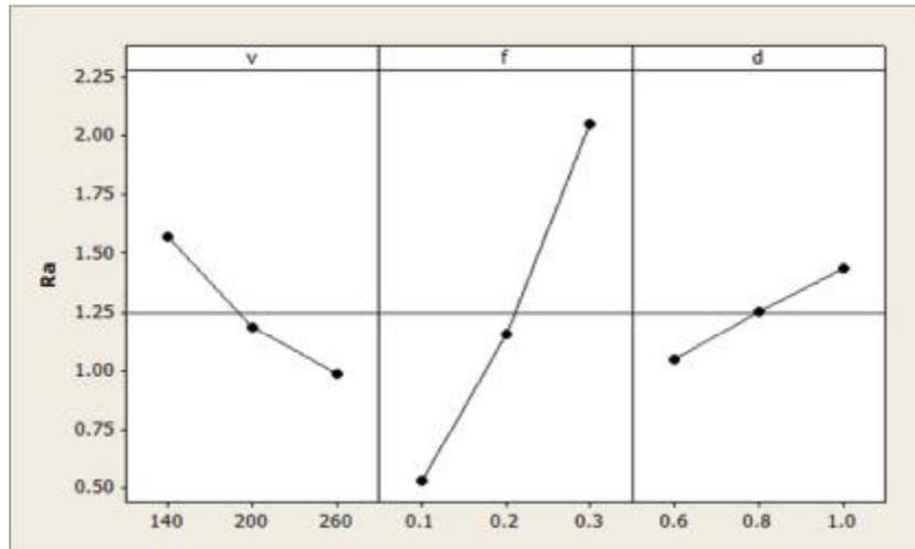
Fig2. Main effect plots for surface roughness (Ra)
