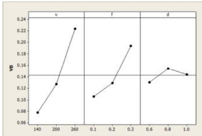
**Fig4.** Main effect plots for flank wear (VB)
