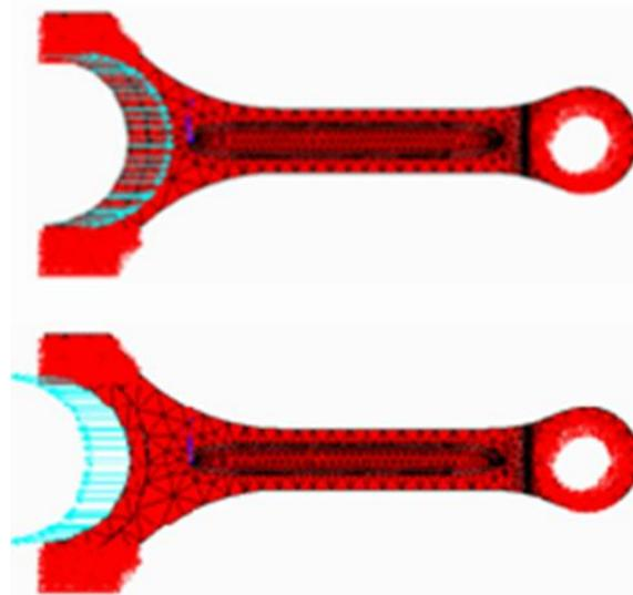
**Fig5.** Compressive (-17,810N) and Tensional (7,870N) Loading.
