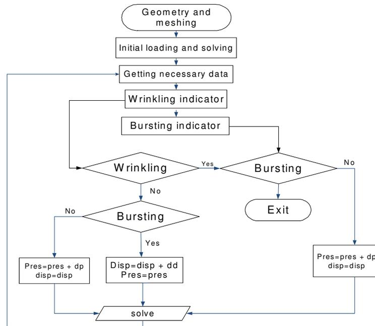
Fig3. The general algorithm of adaptive simulation method
