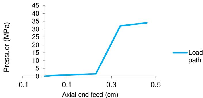
Fig7. Load path determined by adaptive simulation method (present study), tube material DP600 (HG: Z140).
