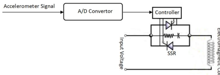
Fig. 8. A schematic diagram for control of the MR mount
