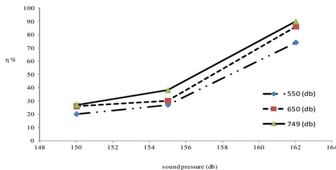
Fig.8. Influence of frequency in acoustic removal efficiency
