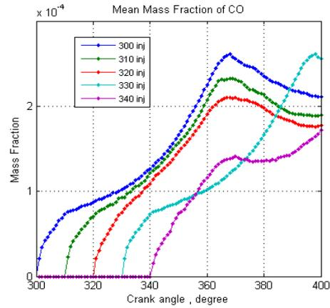
**Fig17.** . Mass fraction of CO versus crank angle
