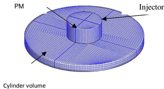
Fig2. Computational mesh for CFD calculation at TDC
