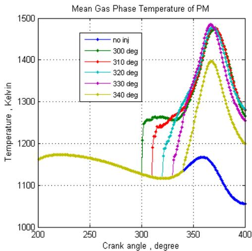
Fig14. Mean temperature distribution in gas phase of PM versus crank angle
