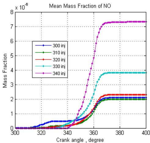
**Fig18.** Figure 18. Mass fraction of NO versus crank angle
