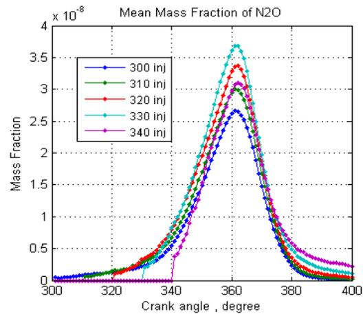
**Fig19.** Figure 19. Mass fraction of N<sub>2</sub>O versus crank angle
