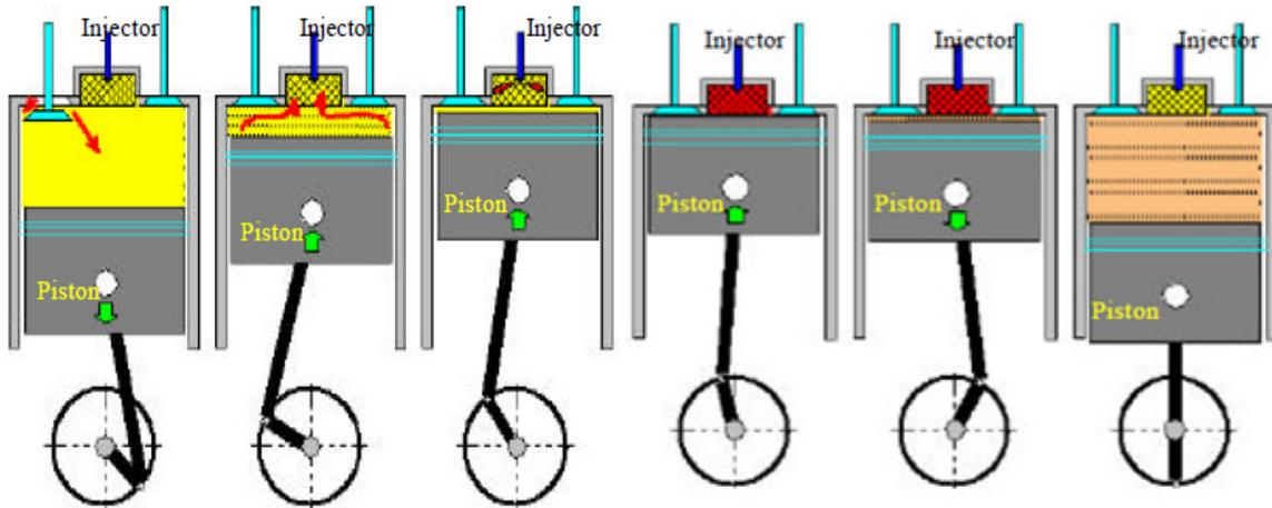
Fig1. A permanent contact PM-engine in operation [10]
