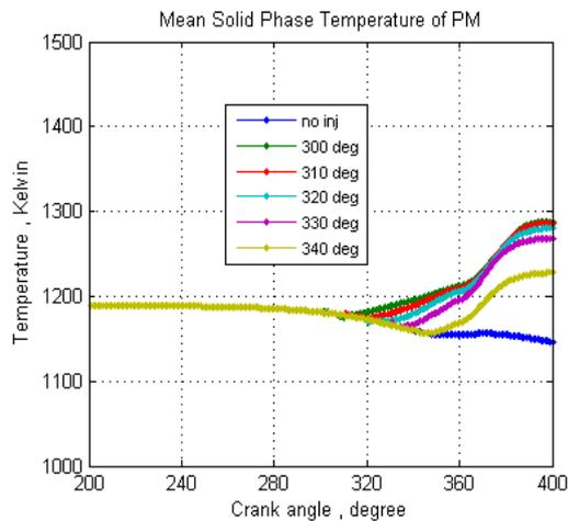
Fig15. Mean temperature distribution in solid phase of PM versus crank angle
