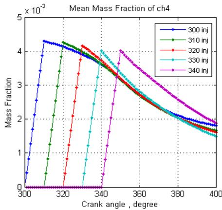
**Fig16.** . Mass fraction of methane versus crank angle
