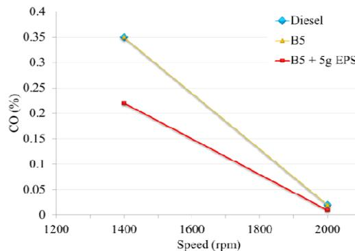
Fig3.CO emission vs. speed at full load
