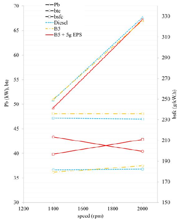
Fig2. Performance parameters vs. speed at full load
